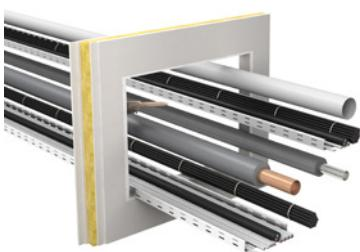
2. Mask the aperture with crepe tape on all sides, keeping 20 mm distance to the edge. Coat the cables with FLAMMOTECT-A; alternatively apply fire protection wrap.
