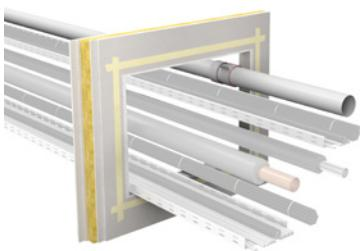
4. Apply the required fire protection wraps to non-combustible pipes.
