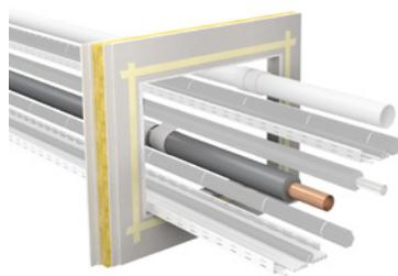
5. Cut mineral fibre boards to size (make cut-outs for the installations).
