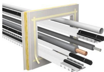
3. Apply fire protection wraps to services, if necessary.
